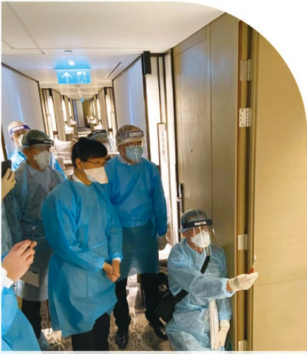
▲ 在指定檢疫酒店調查新型冠狀病毒病群組個案期間進行的煙霧測試 Smoke test conducted during investigation of a cluster of COVID-19 cases in a DQH
